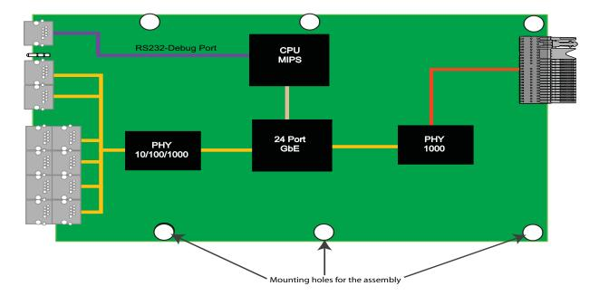
FIGURE 2. VT804 Functional Block Diagram
